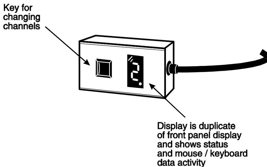
Figure 3 - Remote control pad / display (optional accessory - part RC1)
