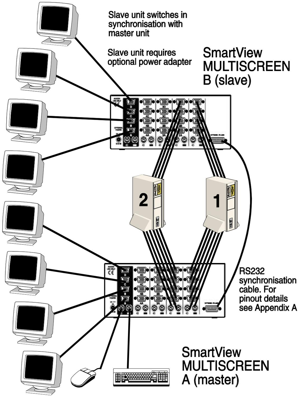
Synchronised SmartView Multiscreens used to switch eight video channels together
