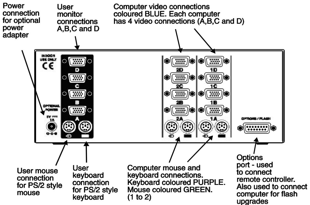
Figure 2c - SmartView Multiscreen rear view (Model SVMS2-Quad)
