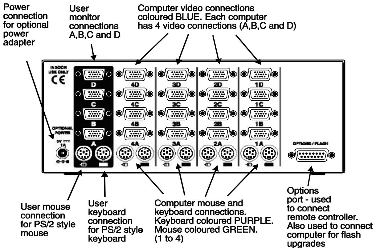
Figure 2a - SmartView Multiscreen rear view (Model SVMS4-Quad)
