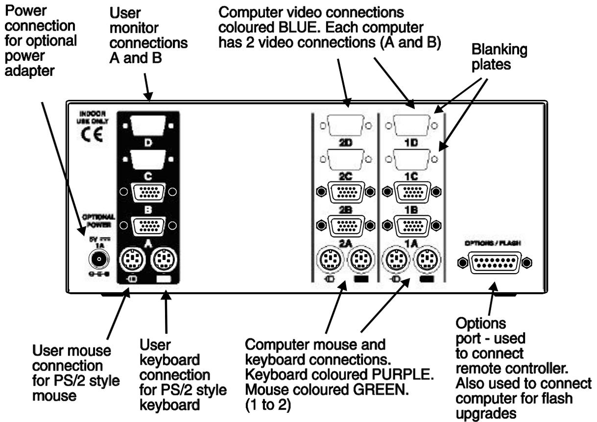
Figure 2d - SmartView Multiscreen rear view (Model SVMS2-Dual)
