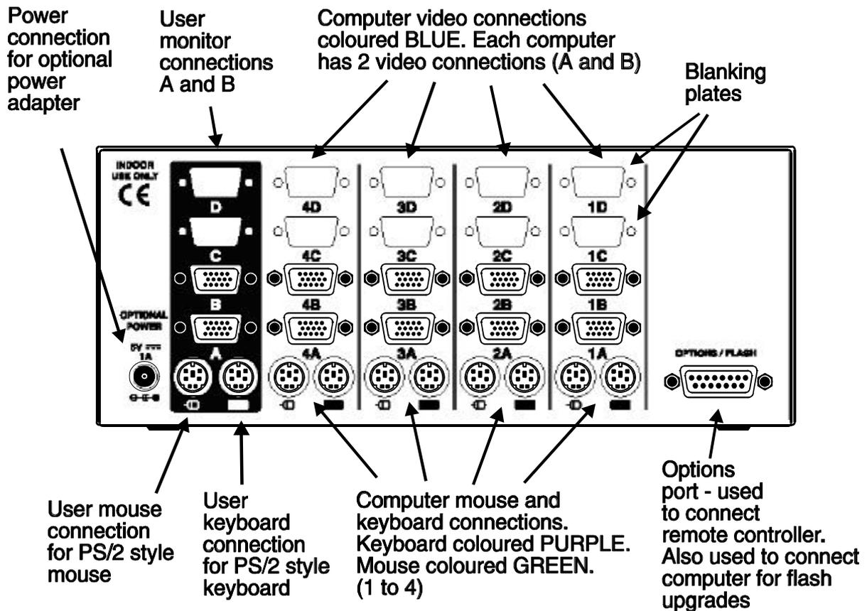
Figure 2b - SmartView Multiscreen rear view (Model SVMS4-Dual)
